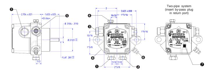
1 Inlet 2 Return 3 Nozzle outlet 4 Pressure gauge port 5 Pressure adjustment 6 Bleeder valve 7 Internal by-pass plug 8 Cone valve
